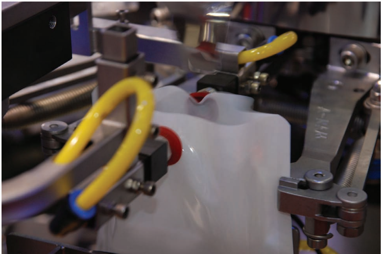
▲ Plastic pack opening / VTEC Bellows Cup - VB20M
