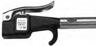
410-SV Parker Venturi Nozzle Controlled Pressure Blow Gun with thumb lever valve and large venturi side ports for high volume flow. Inlet port is 1/4" NPT.
