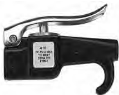
410 Parker two way thumb lever valve has an zinc body with 1/4" NPT inlet and 1/8" NPSF outlet.
