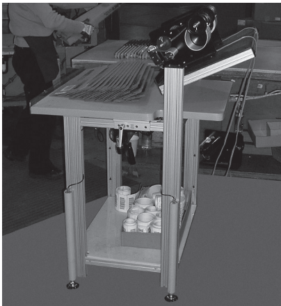
Ergonomic Packaging Table with Lift System and Slide-Out Table Top
