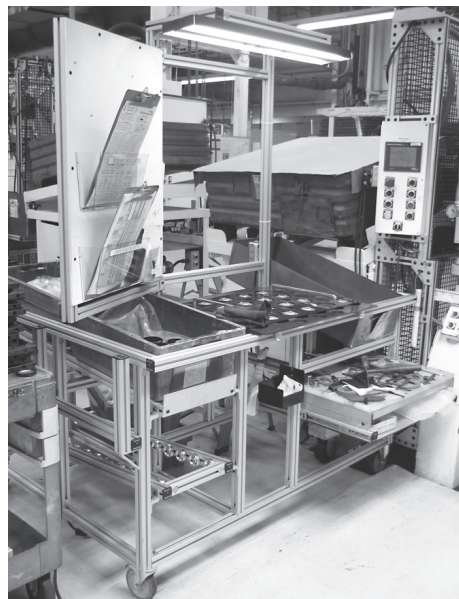
Ultimate Work-cell with Overhead Lighting, Status Board, Gravity Flow Rack, Heavy Duty Pull Out Tool Tray, and Parts Bin on Casters
