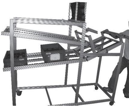
Tote Fill Station and Transfer
