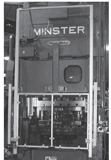
Safety Press Guard with Light Curtains
