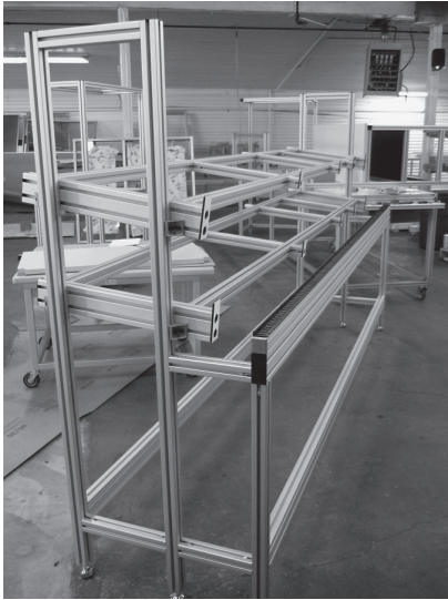
Custom Assembly Station With Rollers
