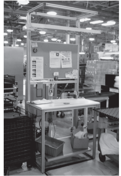
Worktable with Adjustable Shelving on Bottom and Cork Board on Back
