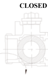
Valve - closed and draining occurs. Upstream seat prevents air flow. Downstream system is vented to atmosphere.
