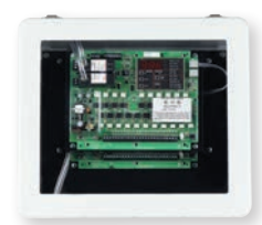
Master board stacked with channel expander
