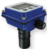
BAT-M shown installed on Series EFS2 meter. Meter sold separately.
