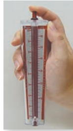
For high scale reading, finger covers hole
