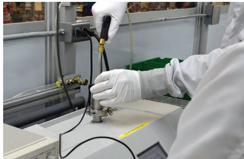
ABOVE: Performing helium leak detection test; BELOW: Custom testing station
